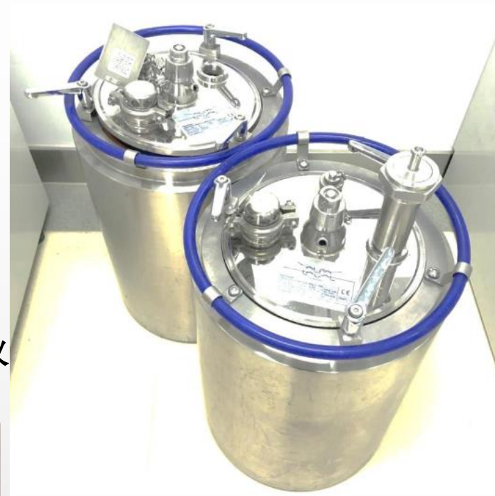
Alfa Laval 实验室酵母扩培设备 Yeast Propagation devices in the lab
